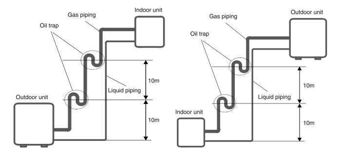
1. Indoor unit is installed higher than outdoor unit 2. Outdoor unit is installed higher than indoor unit.
